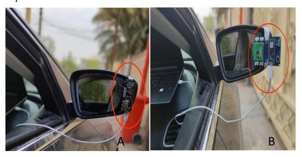
Figure 3.8 (A.) Arduino Portenta H7 test (B.) Arduino Nano 33 BLE test
