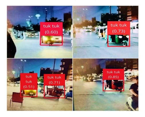
Figure 4.2 Real-time results of work using portent H7 with YOLOv5 algorithm during night-time
