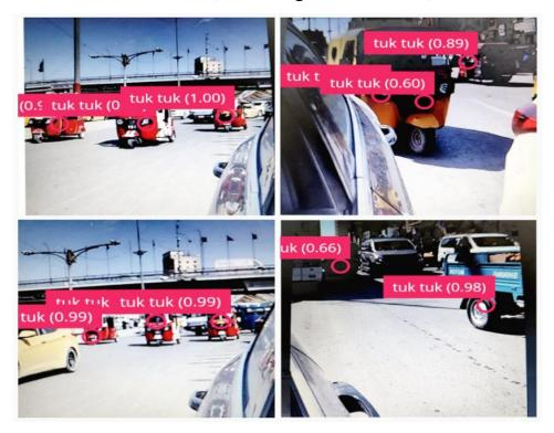
Figure 4.6 Real-time results of work using Portinta H7 with FOMO algorithm and image size 320\*320
