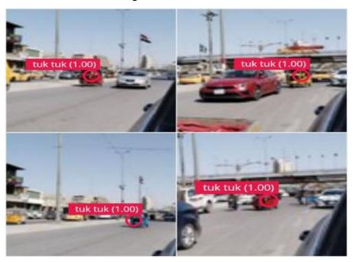
Figure 4.5 Real-time results of work using the OV7675 camera with FOMO algorithm and image size 70\*70
