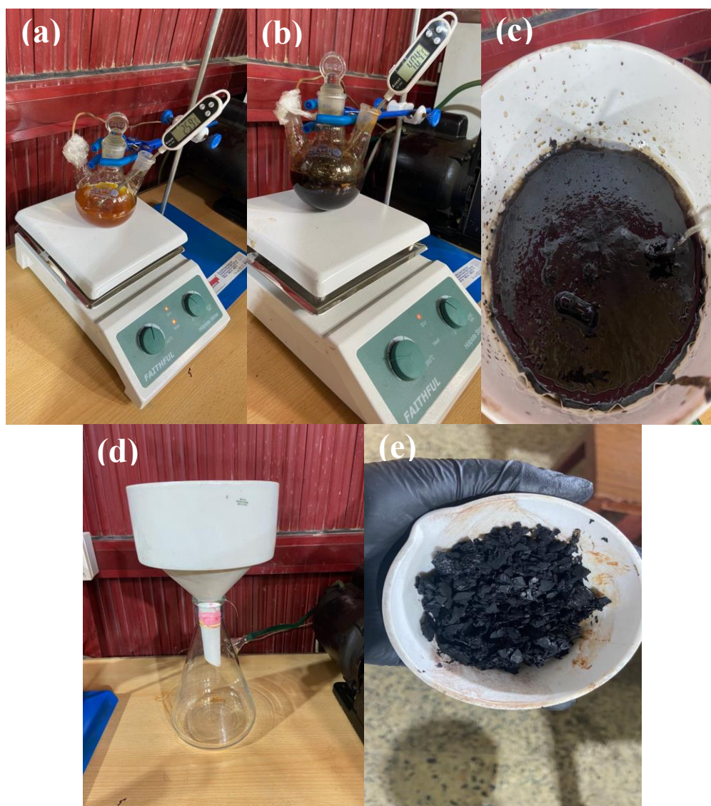
Figure 3-2: Steps for synthesis \text{Fe}_3\text{O}_4 (a) co-precipitation of \text{FeCl}_3 \cdot 6\text{H}_2\text{O} and \text{FeCl}_2 \cdot 4\text{H}_2\text{O} with distilled water. (b) After adding \text{NH}_4\text{OH} and the color changed to black (c) The solid product collected by filter paper. (d) using vacuum pump. (e) \text{Fe}_3\text{O}_4 after removing the residual solvent by oven.
