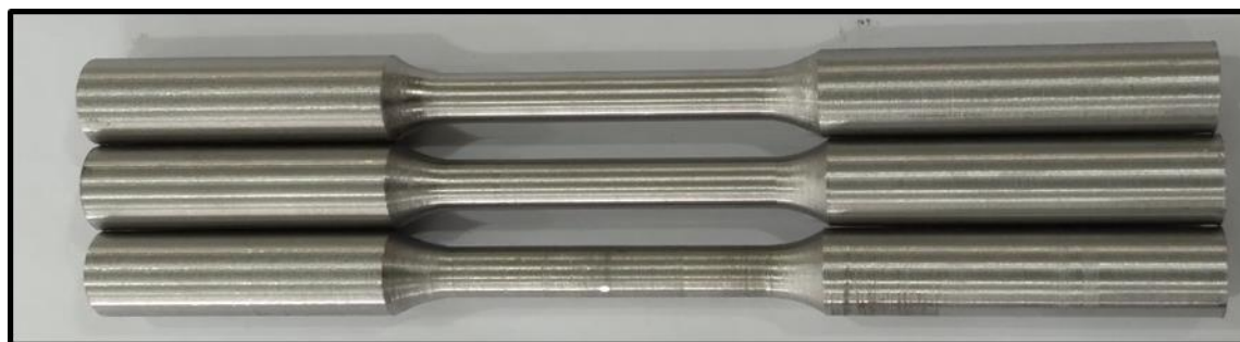
Figure (3.5): Samples of specimens used for tensile test.
