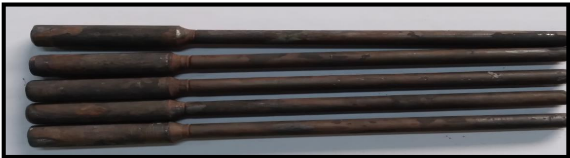
Figure (3.14): Specimen After quenching.
