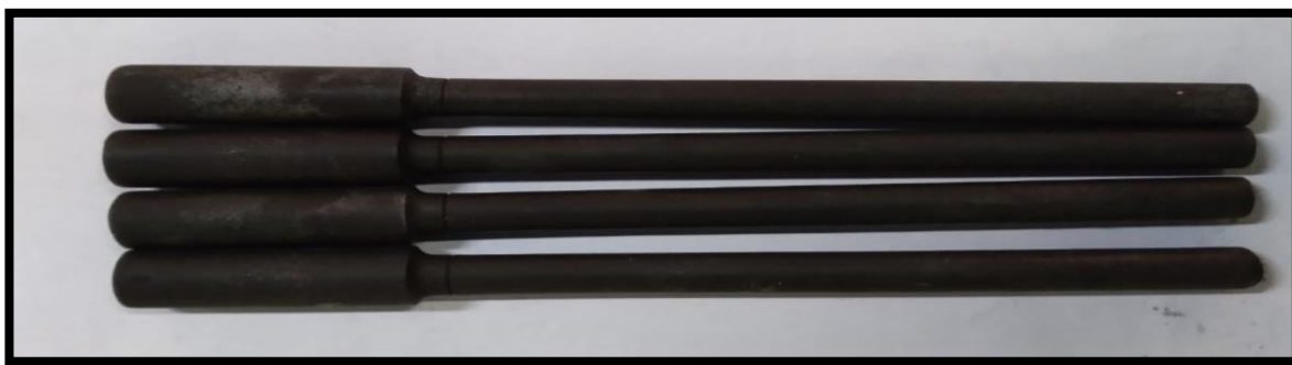
Figure (3.13): Specimens after pack carburizing.
