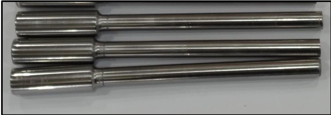
Figure (3.11): Notched Specimens.
